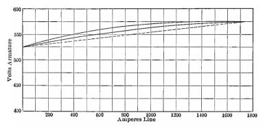
FIG. 88. Commercial compounding curve of d. c. generator (G. E. Co.). Upper line with decreasing load, middle line with increasing load, dash line, perfect over-compounding.
